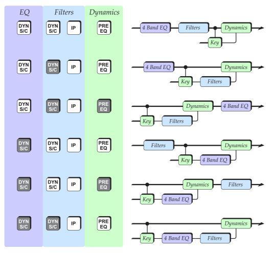
Note that the side chain can be fed from the KEY input on the rear of the unit by selecting KEY.
